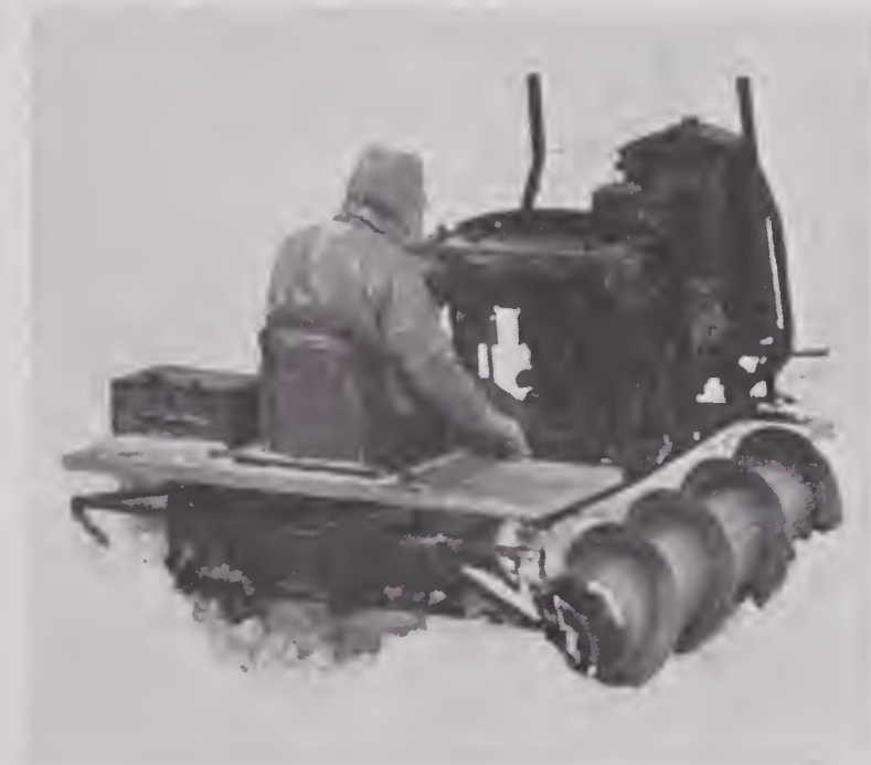
FIGURE 10. Small twin Archimedean screw vehicle digging into soft snow on slight grade.
